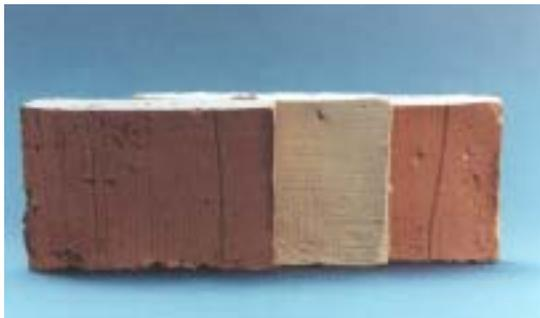
Different baking colours of bricks ( by J.Aarsen).
