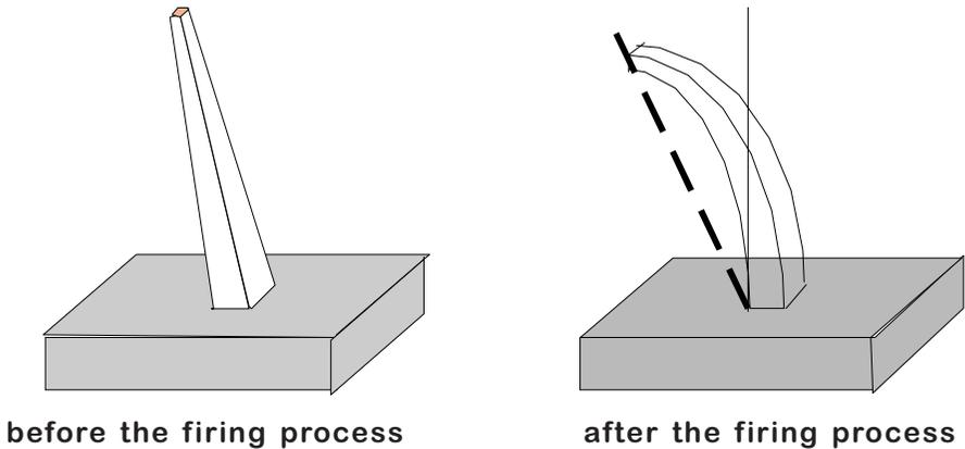
**Fig. 11.3.1** The application of a Seger cone.
