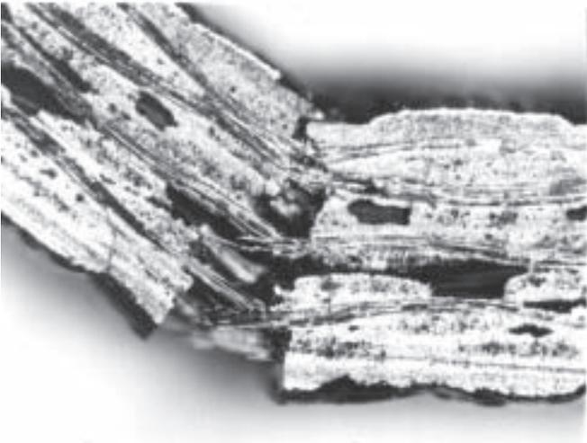
Photo 14.1 / 14.2 Optical micro-photograph of a SiC/SiC<sub>f</sub> composite, made by means of CVI before and after a three point bending test (source: Ube Industries Co Ltd Japan).
