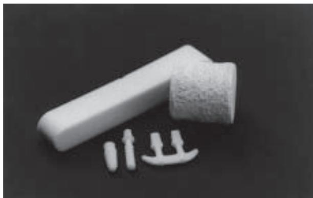
Dense ceramics (bar), porous ceramics (cylinder), teeth anchorings (by : J.Aarsen)
