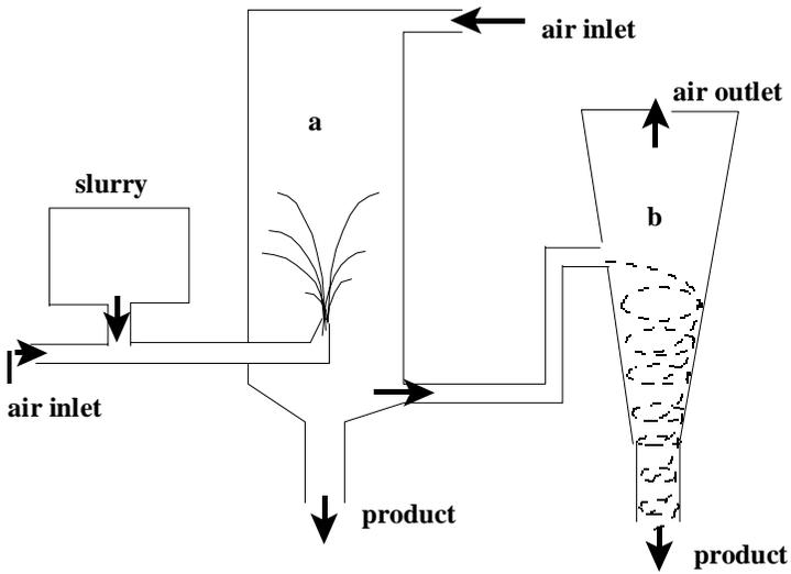
Fig.9.7 Spray drier (a) and cyclone separator (b).
