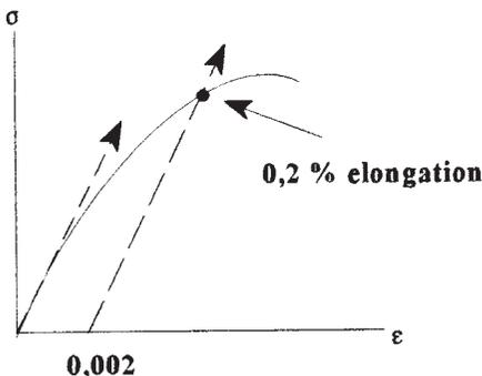
Fig. 10.9 Transition between elastic and plastic deformation (0.2% elastic limit).
