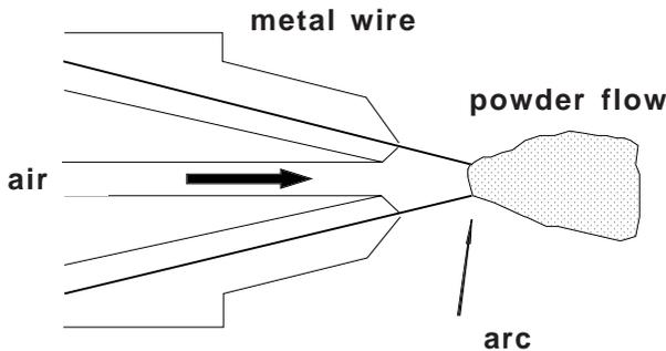
**Fig. 11.7.10** Arc spraying.
