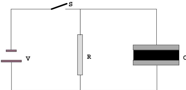
**Fig. 11.4.20** Circuit for the discharge of a capacitor.
