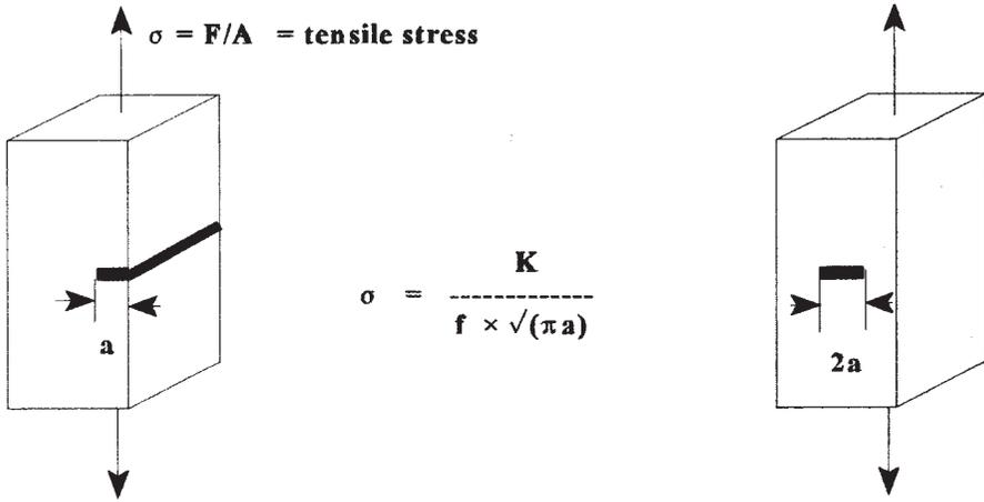
Fig. 9.31 Tensile test of a ceramic sample.
