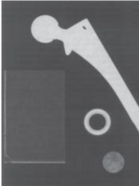
X-ray photograph of a hip joint, a rectangular piece of foam ceramics, a round glass reinforced with titanium fibers and a ring made of metal and ceramics (picture by J Bormans).
