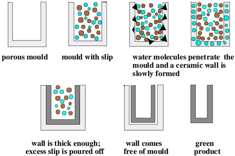
**Fig. 9.21** Slip casting.
