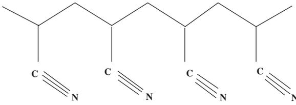
**Fig. 14.4** A polyacrylonitrile chain.
