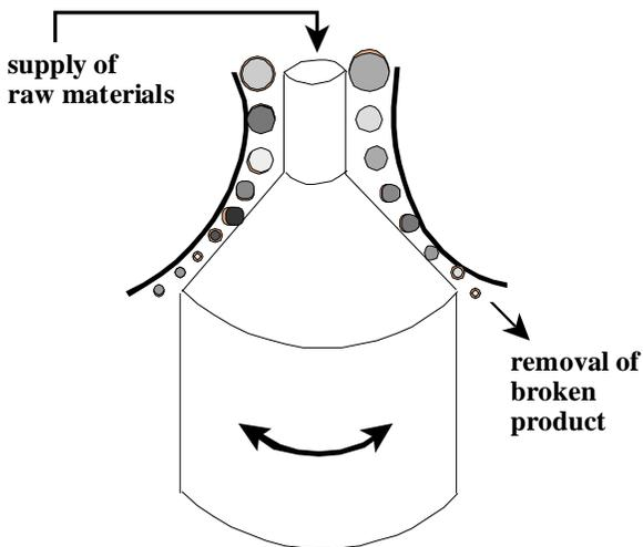
**Fig. 9.5** Conical crusher.
