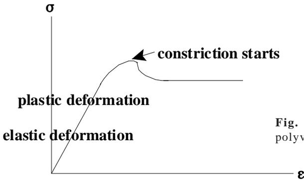
Fig. 10.8 The  $\sigma$ - $\epsilon$  curve of polyvinyl chloride PVC.
