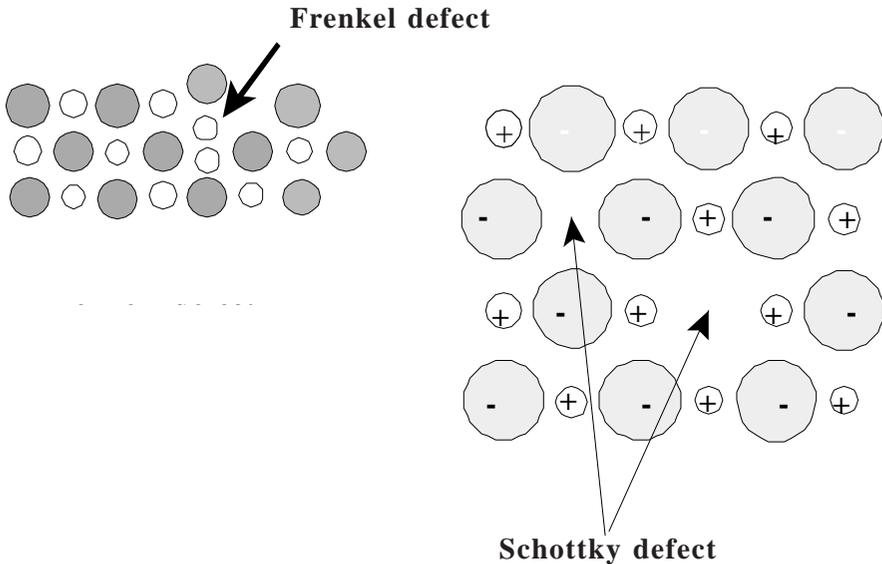
Fig. 4.8 Point defects.
