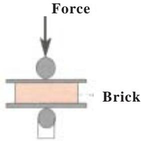
**Fig. 11.2.3** Measuring the fracture strength of a brick.
