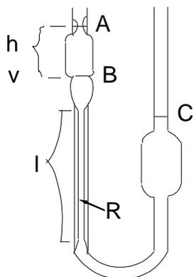
**Fig. 5.10** Ostwald viscometer.
