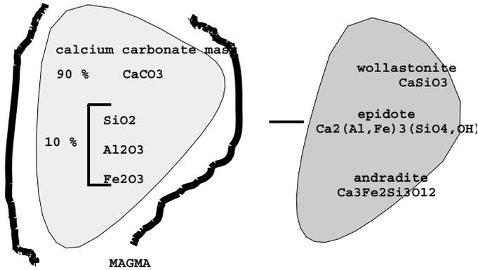
Fig. 7.4 An example of a metamorphic process.
