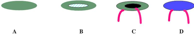
**Fig. 11.4.21** The construction of a ceramic capacitor.
