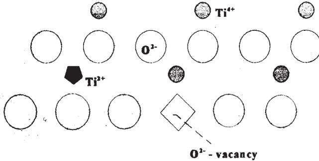
**Fig. 11.7.6** A  $\text{TiO}_2$  crystal with  $\text{O}^{2-}$  vacancies.
