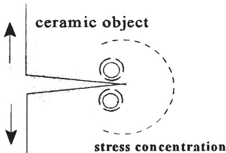
**Fig. 14.8** Preventing the expansion of a crack by incorporating zirconium particles.
