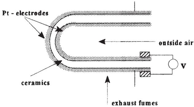
Fig. 11.7.4 Extremely schematic representation of the lambda-probe.
